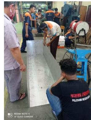
Gambar 6. Proses assembly tabung ketel
