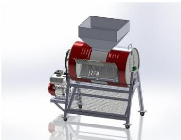
**Gambar 2.** Design Mesin Corn Sheller
