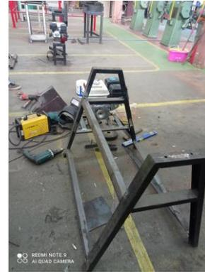
**Gambar 4.** Rangka Mesin Corn Sheller
