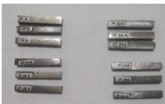
**Gambar 2.** Specimen Uji Impact ASTM E23
