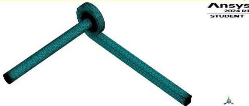
Gambar 4. Hasil Mesh Centrifugal Fan
