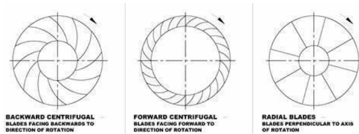
Gambar 2. Tipe Impeller (Mahmoodi-Eshkaftaki & Ebrahimi, 2019)
