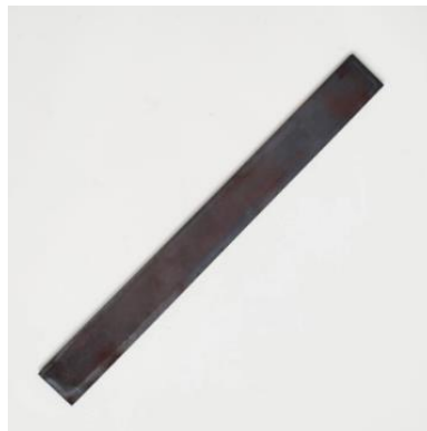
Figure 1 ASTM 440C steel before cut and before ground
